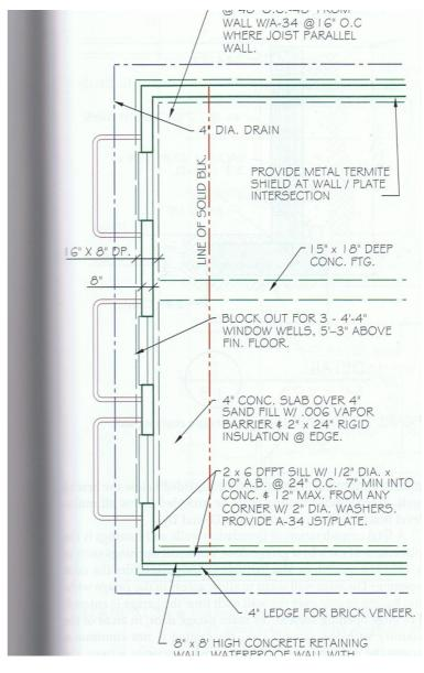
The code further states that if the escape or rescue window finished sill height is below the adjacent ground level (as it would normally be in a basement) it shall have a window well (areaway). The window well or areaway must have a minimum net clear opening of 9 square feet, With a minimum horizontal dimension of 3 feet.
