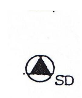
The code requires the smoke detector to be connected to the normal electrical wiring as well as having a battery-powered backup system.
