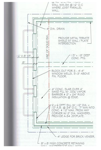
If the window well has a vertical depth of more than 44 inches it shall be provided with an approved permanently affixed ladder. This ladder cannot encroach into the 9 foot minimum area more than 6 inches.
