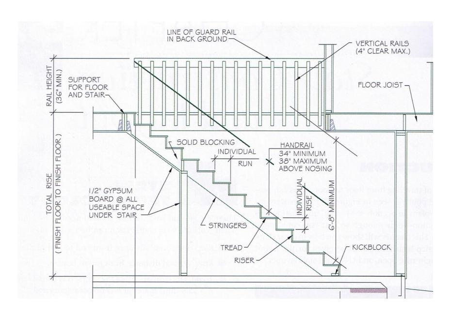
The railings must be constructed so that a 4 inch diameter sphere cannot pass through any opening in the rail.
