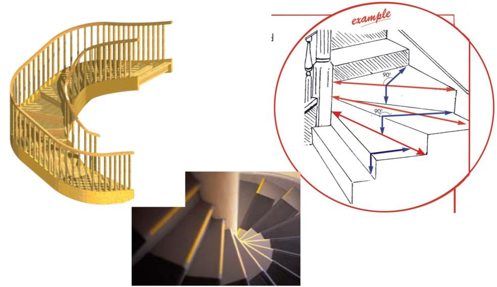
The code provides a variation on minimum tread and maximum riser dimensions for spiral stairs.
