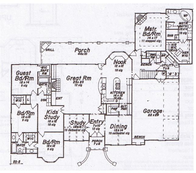
The kitchen is not required to meet the habitable room lighting and ventilation requirements.
