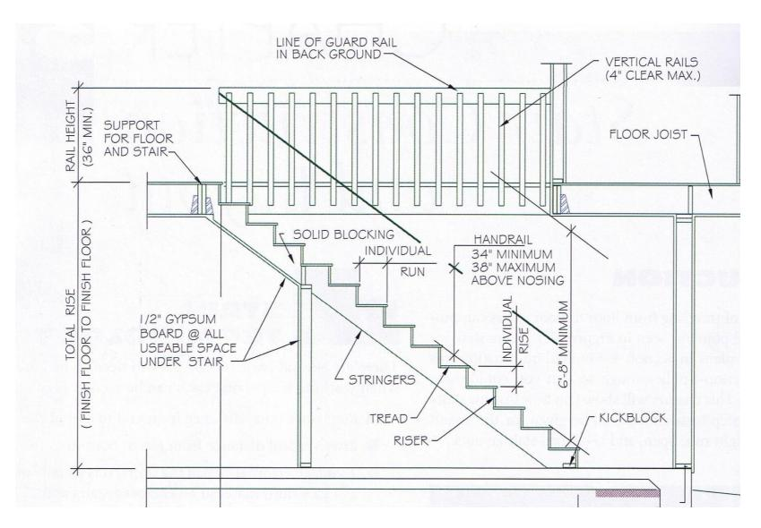
If there is any variation in riser height or in tread run on a flight of stairs, the difference between the largest and smallest cannot exceed 3/8 inch.
