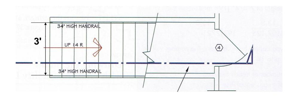
Common stair tread lengths should be between 10 inches and 10  $\frac{1}{2}$  inches with a rise of about 7  $\frac{1}{2}$  inches.
