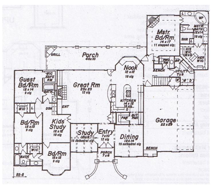
Every dwelling unit is required to have at least one room with a minimum area of 150 square feet. All other habitable rooms must have a minimum area of 70 square feet. The minimum wall to wall distance is a habitable room is 7 feet.
