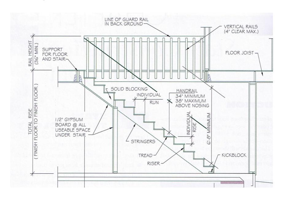
The code requires the top of the handrail to be between 34 and 38 inches above the nose of the tread.
