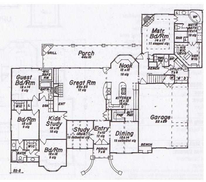
Smoke detectors must be located in each sleeping room as well as a point centrally located in the corridor providing access to the bedroom.
