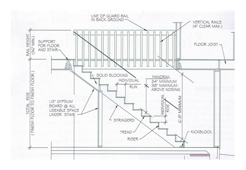
The guardrail must be provided at any change in floor elevation that exceeds 30 inches.
