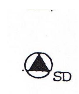
The smoke detectors must be interconnected in such a way that when one alarm is activated they all sound.
