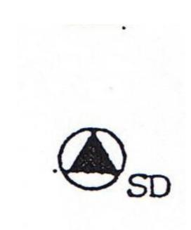
The code states that, when the dwelling unit has more than one story and in dwellings with basements, a detector shall be installed on each story and in the basement.
