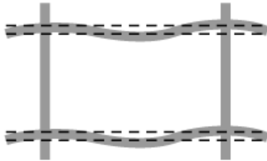
floor slab deflection (non-cyclical)
