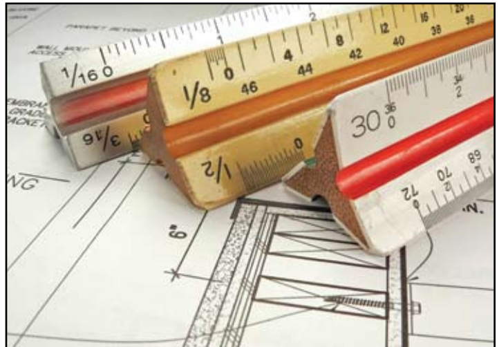
Typical Scales Used by Drafters
